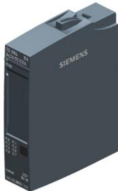
SIPLUS ET 200SP DQ 8x24V DC/0.5A Sink Basic based on 6ES7132-6BF61-0AA0 with conformal coating, -40...+70 °C, digital output module, suitable for BU type A0, color code CC01
