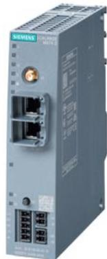
SCALANCE M874-3 3G router; for wireless IP communication from Ethernet-based programmable controllers via 3G mobile radio HSPA+, VPN, firewall, NAT; 2-port switch; 1x digital input, 1x digital output; observe national approvals.
