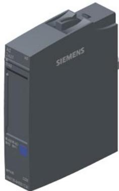
SIPLUS ET 200SP AQ 2xU/I HF based on 6ES7135-6HB00-0CA1 with conformal coating, -40...+70 °C, analog output module, suitable for BU type A0, A1, color code CC00, channel diagnostics, 16-bit, +/-0.1%
