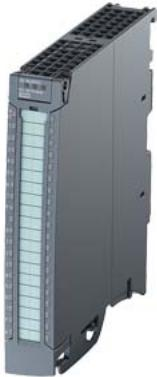
SIMATIC S7-1500, digital output module, DQ16xDC 24V/0.5A BA, 16 channels in groups of 8, 4 A per group; the module supports the safety-oriented shutdown of load groups up to SIL2 according to EN IEC 62061:2021 and Category 3 / PL d according to EN ISO 13849-1:2015. delivery incl. front connector push-in
