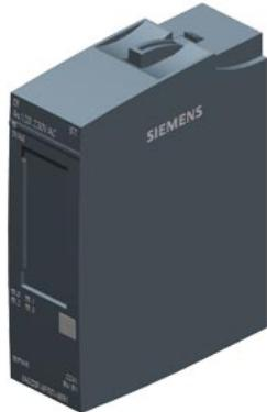
SIPLUS ET 200SP DI 4x120/230VAC TX rail based on 6ES7131-6FD01-0BB1 with conformal coating, -40...+70 °C, OT4 with ST1/2 (+85 °C for 10 minutes), digital input module, suitable for BU type B1, color code CC41, module diagnostics input type 3 (IEC 61131),
