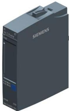
SIPLUS ET 200SP AI 4xI 2-/4-wire standard based on 6ES7134-6GD01-0BA1 with conformal coating, -40...+70 °C, analog input module, suitable for BU type A0, A1, color code CC03, module diagnostics, 16-bit, +/-0.3%
