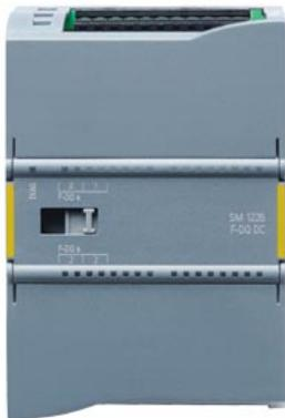
SIPLUS S7-1200 SM 1226 F-DQ 4x24VDC based on 6ES7226-6DA32-0XB0 with conformal coating, -25...+55 °C, F-DQ 4x DC 24V 2A, PROFIsafe, 70 mm width, up to PL e (ISO 13849-1)/ SIL3 (IEC 61508)
