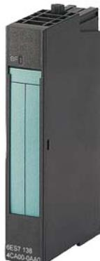
SIMATIC DP, Electronics module ET 200S 4AI standard I-2-wire, 4-20 mA; 13 bit, 15 mm width, for 2-wire transducer Cycle time 40 ms/module with SF LED (group fault)
