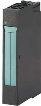
SIPLUS ET 200S EM 2AQ I standard based on 6ES7135-4GB01-0AB0 with conformal coating, -25...+70 °C, +/-20 mA; 13 bit+sign, 4..20 mA; 13 bit cycle time less than 1 ms with SF LED (group fault)
