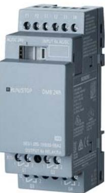
LOGO! DM8 24R expansion module, PS/I/O: 24V/24V/relay, 2 MW 4 DI/4 DO, AC/DC/NPN input for LOGO! 8
