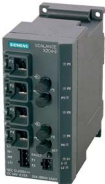
SCALANCE X204-2, managed IE switch, 4x 10/100 Mbit/s RJ45 ports, 2x 100 Mbit/s multimode BFOC, LED diagnostics, error signaling contact with set pushbutton, redundant power supply, PROFINET IO device, network management; Redundancy Manager integrated, incl. electron. manual on CD-ROM, C-PLUG optional.
