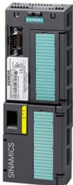
SIPLUS G120 CU240E-2 DP based on 6SL3244-0BB12-1PA1 with conformal coating, -20...+55 °C, Control Unit CU240E-2 DP E-type with Safety Integrated STO PROFIBUS DP 6 DI, 3 DQ, 2 AI, 2 AQ, max. 1F-DI PTC/KTY interface USB and SD/MMC interface degree of protection IP20 ambient temperature 0 to +50 °C without Power Module
