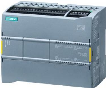
SIPLUS S7-1200 CPU 1215FC DC/DC/DC based on 6ES7215-1AF40-0XB0 with conformal coating, -25...+55 °C, compact CPU, DC/DC/DC, 2 PROFINET ports, onboard I/O: 14 DI 24 V DC; 10 DQ 24 V DC 0.5 A; 2 AI 0-10 V DC, 2 AQ 0-20 mA DC, power supply: DC 20.4 - 28.8 V DC, program/data memory 150 KB
