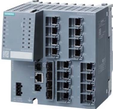
SCALANCE XM416-4C; managed modular IE switch; 16x 10/100/1000 Mbit/s RJ45; 4x 100/1000 Mbit/s SFP; contains 4 combo ports; in total 16 ports can be used; expandable to 24 ports electrical or optical; assembly: DIN rail/S7 mounting rail, PROFINET IO device; redundancy functions; office features (RSTP, VLAN, IGMP,..); C-PLUG in scope of supply; layer 3 with Key-Plug plug available .
