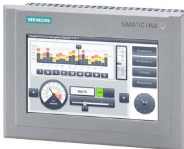
SIMATIC HMI TP700 Comfort Outdoor, Comfort Panel, touch operation, 7" widescreen TFT display, 16 million colors, PROFINET interface, MPI/PROFIBUS DP interface, 12 MB configuration memory, Windows CE 6.0 (Microsoft support including security updates discontinued) configurable from WinCC Comfort V13 SP1, HSP
