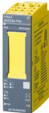
SIMATIC DP, POWER M. F-PM-E PPM PROFIsafe, for ET 200SP; 24 V DC safe shutdown of DQ and F-DQ up to PL D/SIL2 or PL E/SIL3 2 for safe dig. inputs 1 for safe dig. output PPM
