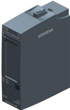
SIPLUS ET 200SP RQ 4x120VDC/230 TX rail based on 6ES7132-6HD01-0BB1 with conformal coating, -40...+70 °C, OT4 with ST1/2 (+85 °C for 10 minutes), relay module normally open, suitable for BU type B0 or B1, color code CC40, substitute value output, module diagnostics for: supply voltage
