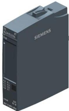
SIMATIC ET 200SP, Digital output module, DQ 8x 24V DC/0,5A Standard, Source output (PNP,P-switching) Packing unit: 10 pieces, fits to BU-type A0, Colour Code CC02, substitute value output, module diagnostics for: short-circuit to L+ and ground, wire break, supply voltage
