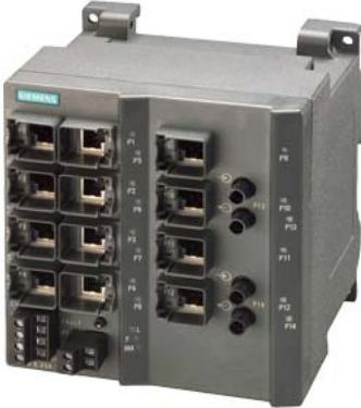
\*\*\*spare part\*\*\* SIPLUS NET SCALANCE X212-2 based on 6GK5212-2BB00-2AA3 with conformal coating, -40...+60 °C, managed IE switch, 12x 10/100Mbps RJ45 ports, 2x 100 Mbps multimode BFOC, LED diagnostics, error signaling contact with set pushbutton, Redundant power supply, PROFINET IO device, network management, integrated redundancy manager, incl. electronic manual on CD-ROM, C-Plug optional
