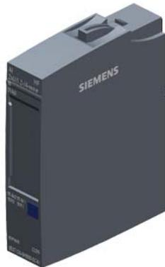
SIMATIC ET 200SP, Analog input module, AI 2x U/I 2.-4-wire High Feat., suitable for BU type A0, A1, Color code CC05, channel diagnostics, 16 bit, +/-0.1%
