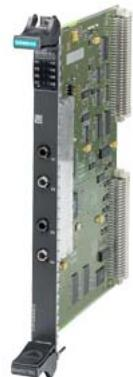
SIMATIC TDC communication module CP 53M0 Rack coupling TDC <-->
