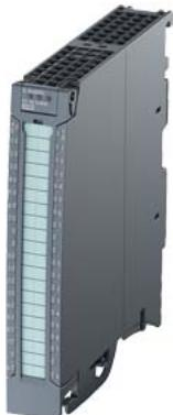
SIMATIC S7-1500 Digital input module, DI 32x24 V DC BA, 32 channels in groups of 16, Input delay typ. 3.2 ms, Input type 3 (IEC 61131); Delivery incl. front connector Push-in
