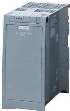
\*\*\*spare part\*\*\* SIPLUS S7-1500 CPU 1516F-3 PN/DP T1 rail based on 6ES7516-3FN01-0AB0 with conformal coating, -25...+60 °C, OT1 with ST1/2 (+70 °C für 10 minutes), central processing unit without display with work memory 1.5 MB for program and 5 MB for data, 1st interface: PROFINET IRT with 2-port switch, 2nd interface: PROFINET RT, 3rd interface: PROFIBUS, 10 ns bit performance, SIMATIC Memory Card required
