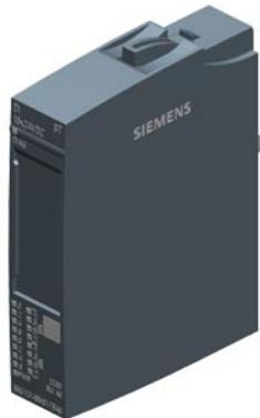
SIPLUS ET 200SP DI 16x24 V DC standard based on 6ES7131-6BH01-0BA0 with conformal coating, -40...+70 °C, digital input module, suitable for BU type A0, color code CC00, type 3 (IEC 61131) sink input, (PNP, sinking input), input delay 0.05..20 ms module diagnostics for: wire break, supply voltage
