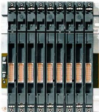
SIMATIC S7-400, extension rack ER2 with 9 slots, only for signal modules
