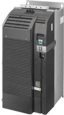
SIPLUS G120 PM240-2 IP20-FSF-U-400V 132 kW based on 6SL3210-1PE32-5UL0 with conformal coating, -20...+50 °C, unfiltered with integrated braking chopper 380-480 V 3 AC +10/-20% 47-63 Hz power high overload: 110 kW at 200% 3 s, 150% 57 s, 100% 240 s power rating low overload: 132 kW at 150% 3 s, 110% 57 s, 100% 240 s 708x305x357 (HxWxD), FSF design, degree of protection IP20 without CU and operating unit released as of CU FW version V4.7 HF8
