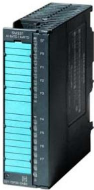
SIMATIC S7, analog input SM 331, isolated, 8 AI thermocouples/4 AI Pt100, for signals from the hazardous area, diagnostics-capable, PTB tested 1 x 20-pole
