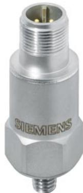
SIPLUS CMS2000 VIB-Sensor S01 Vibration sensor; Frequency range 0.5 Hz to 15 kHz; Measuring range 50G; Sensitivity 100 mV/G (+/-10%); MIL connector on top
