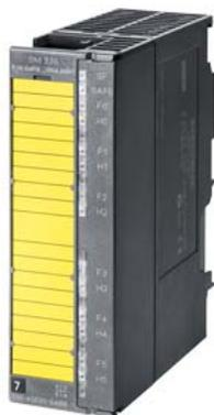
SIMATIC S7, Analog input SM 336, 6 AI; 15 bit; fail-safe analog inputs for SIMATIC Safety, with HART support, up to Category 4 (EN 954-1)/ SIL3 (IEC61508)/PLE (ISO13849), 1x 20-pole
