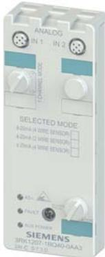
SIPLUS AS Interface 2 AI IP67 based on 3RK1207-1BQ40-0AA3 with conformal coating, -25...+70 °C, AS-Interface compact module, IP67 analog, 2 AI, number format S7, 2x inputs (M12), 4...20 mA for 4-wire sensors active channels 1 and 2 no smoothing filter 50 Hz mounting plate 3RK1901-0CA00 must be ordered separately, profile 7.3
