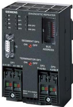
SIMATIC S7, Diagnostic repeaters for PROFIBUS DP, for online diagnostics of the PROFIBUS cable, DP standard slave up to 12 Mbit/s, Degree of protection IP20, FastConnect connection method
