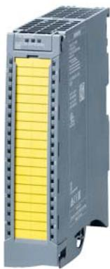
SIPLUS S7-1500 F-DQ 8x24VDC/2A based on 6ES7526-2BF00-0AB0 with conformal coating, -30...+60 °C, F digital output module, 35 mm overall width; up to PL E (ISO 13849-1)/ SIL3 (IEC 61508)
