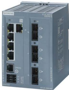
SCALANCE XB205-3 managed Layer 2 IE switch 5x 10/100 Mbit/s RJ45 ports 3x MM FO SC-port 1x console port, diagnostics LED redundant power supply; IEC 62443-4-2 certified; temperature range 0 °C to +60 °C; DIN-rail mounting; default PROFINET.
