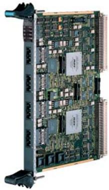
SIMATIC TDC Communication module CP 52IO Interface module for Global Data Memory (GDM) with 4 interfaces
