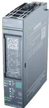
\*\*\* spare part \*\*\* SIPLUS ET 200SP TM Posinput 1 based on 6ES7138-6BA00-0BA0 with conformal coating, -40...+60 °C, counting and position detection module for RS-422 incremental encoder or SSI absolute encoder, 2 DI, 2 DQ suitable for BU type A0,
