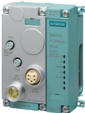
SIMATIC DP, PROFINET Interface module IM 154-3 PN, High Feature for ET 200 PRO, Integrated switch, incl. termination module, Connection modules 6ES7194-4AK00-0AA0 order separately
