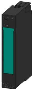
SIMATIC DP, Electronics module for ET 200S, 2/4 AI RTD Standard, 15 mm width, 15 bit+sign Pt100 STD; Pt100 KL; NI100 STD; NI100 KL; 150 ohm; 300 ohm; 600 ohm; Cycle time 110 ms/channel with SF LED (group fault)
