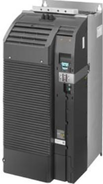
SIPLUS G120 PM240-2 IP20-FSF-A-400V 75 kW based on 6SL3210-1PE31-5AL0 with conformal coating, -20...+50 °C, with integrated class A filter with integrated braking chopper 380-480 V 3 AC +10/-20% 47-63 Hz power high overload: 55 kW at 200% 3 s, 150% 57 s, 100% 240 s power low overload: 75 kW at 150% 3 s, 110% 57 s, 100% 240 s 708x 305x 357 (HxWxD), FSF design, degree of protection IP20 without CU and operating unit released as of CU FW version V4.7 HF8
