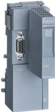
SIMATIC DP, CM PROFIBUS DP for ET 200SP CPU module with PROFIBUS DP interface (9-pole D-sub socket) DP master for 125 DP slaves DP slave,
