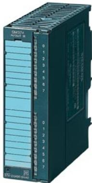
SIMATIC S7-300, Simulator module SM 374, for simulation of 16 inputs or 16 outputs or 8 inputs and 8 outputs 16 switches, 16 LEDs
