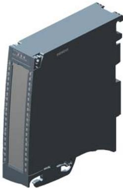
SIPLUS S7-1500 TM Posinput 2 based on 6ES7551-1AB00-0AB0 with conformal coating, -25...+70 °C, counting and position feedback module, 2 channels, for RS-422 incremental encoder or SSI absolute encoder, 2 DI, 2 DQ per channel
