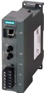
SIPLUS NET SCALANCE X101-1 based on 6GK5101-1BB00-2AA3 with conformal coating, -10...+60 °C,
