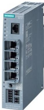
SCALANCE M816-1 ADSL router; for wire-bound IP communication from Ethernet-based automation devices via Internet service provider; VPN, Firewall, NAT; 4-port switch; 1x digital input, 1x digital output; ADSL2+, Annex A .
