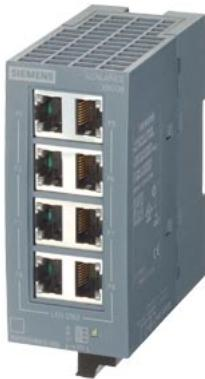
\*\*\*\*\* spare part \*\*\*\*\* SCALANCE XB008 unmanaged Industrial Ethernet Switch for 10/100 Mbit/s; for setting up small star and line topologies; LED diagnostics, IP20, 24 V DC power supply, with 8x 10/100 Mbit/s twisted pair ports with RJ45 sockets; manual available as a download .
