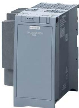
SIPLUS S7-1500 CPU 1516-3 PN/DP TX rail based on 6ES7516-3AN01-0AB0 with conformal coating, -40...+70 °C, OT4 with ST1/2 (+85 °C for 10 minutes), heat sink, no PS usable, central processing unit without display with work memory 1 MB for program and 5 MB for data, 1st interface: PROFINET IRT with 2-port switch, 2nd interface: PROFINET RT, 3rd interface: PROFIBUS, 10 ns bit performance, SIMATIC Memory Card required
