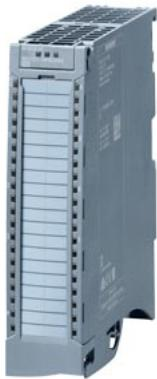
SIPLUS S7-1500 AI 8xU/I HF based on 6ES7531-7NF00-0AB0 with conformal coating, -40...+70 °C, start up -25 °C, analog input module 16-bit resolution, accuracy 0.1%, 8 channels in groups of 1, common mode voltage: 30 V AC/60 V DC, diagnostics; hardware interrupts; including infeed element, shielding bracket and shield terminal
