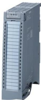
SIMATIC S7-1500, digital input module DI 16xNAMUR HF, 16 channels in groups of 8; for 8.2 V NAMUR encoder; sensor supply 8.2 V; input delay; parameterizable 0.05 ... 20 ms; integrated counting function up to 20 kHz pulse stretching; chatter monitoring; signal inversion diagnostics; hardware interrupts; all necessary components for shielding included in the scope of supply; front connector (screw terminals or push-in) to be ordered separately
