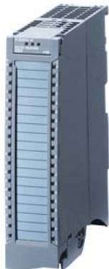
SIMATIC S7-1500, digital input module DI 16x24 V DC HF, 16 channels in groups of 16; of which 2 inputs as counters can be used; input delay 0.05..20 ms; input type 3 (IEC 61131); diagnostics; hardware interrupts: front connector (screw terminals or push-in) to be ordered separately
