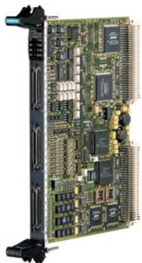
SIMATIC TDC Signal module SM500 with 8 AO/8 AI/16 DO/16 DI/ 4 incremental encoder inputs/ 4 absolute value encoder inputs/ 6 LEDs
