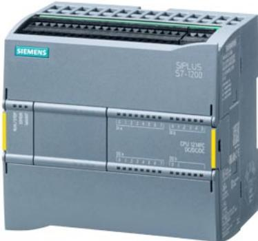
SIPLUS S7-1200 CPU 1214FC DC/DC/relay based on 6ES7214-1HF40-0XB0 with conformal coating, -25...+55 °C, compact CPU, DC/DC/relay, onboard I/O: 14 DI 24 V DC; 10 DQ relay 2 A; 2 AI 0-10 V DC, power supply: DC 20.4-28.8 V DC, program/data memory 125 KB
